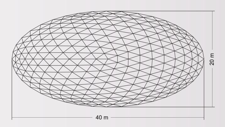
base area: 1256 sq/m base diameter: 40m dome height: 14m setup time: 7 days
